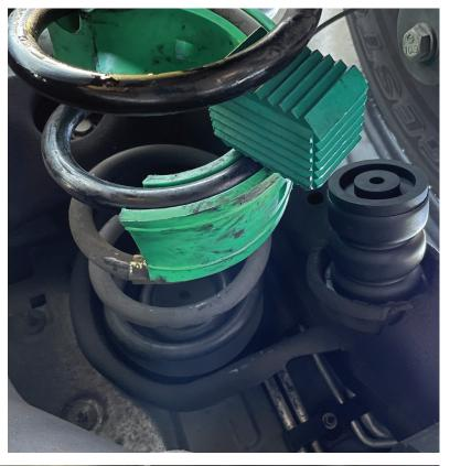
Adding two MUB2 on MUB1A as the cushion between frame and axel Add another 0.5" ground clearance to 39"
