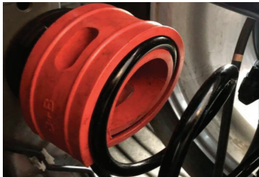
2019 Honda CRV Size : A+ (Front) , B (Rear) Ground Lifting Height : 1.2"
