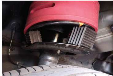
2018 Mitsubishi Outlander Size : A (Front) , D & E (Rear) Ground Lifting Height : Up ~1.5"
