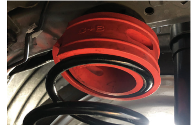
2019 Honda HR-V LX Size : A (Front) , B+ (Rear) Ground Lifting Height : 1.2"
