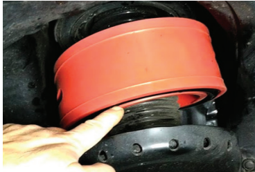
2017 Subaru Crosstrek Size : A (Front) , D (Rear) Ground Lifting Height : 1"
