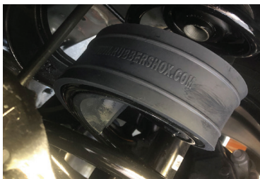
2019 Mazda 6 Size : B+ (Front) , B+ (Rear) Ground Lifting Height : 0.75"
