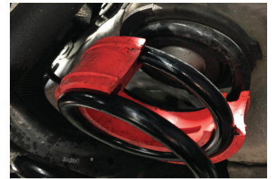
2013 Honda Civic Size : C (Front) , D (Rear) Ground Lifting Height : 0.7"
