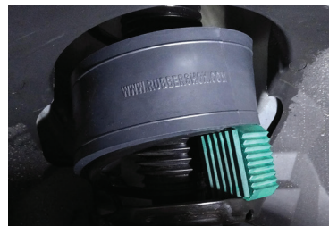
2019 Volvo XC40 Size : A+ (Front) , DuraShock Block (Green) : Adds extra 0.5" Total Ground Lifting Height : 1.7"
