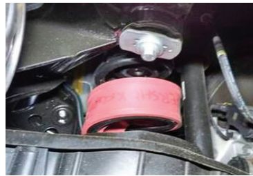
2020 Volvo XC40 Size : A (Front) , B (Rear) Ground Lifting Height : Up ~1.5"
