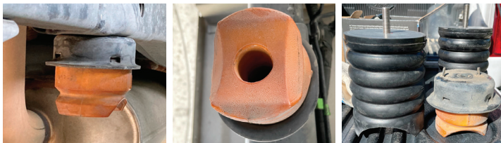
Remove Original Factory Bump Stops with M16 Socket
