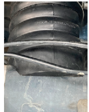
Curved Surface will sit on Axle after Loading
