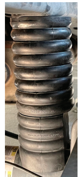
Adding one extra UB2 into UB1223A 8.5" Height
