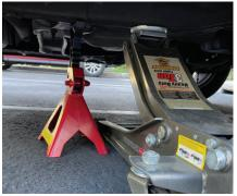
1.Jack up the SUV and put safety lift stop.
