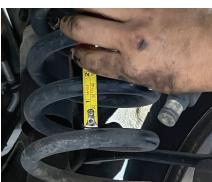
2. The measurement of the spring gap was 1.1" so CSBPlus-D size D and RB125-1-1 were selected.
