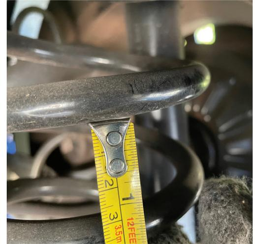
5. The rear coil springs gap is around 1.1".
