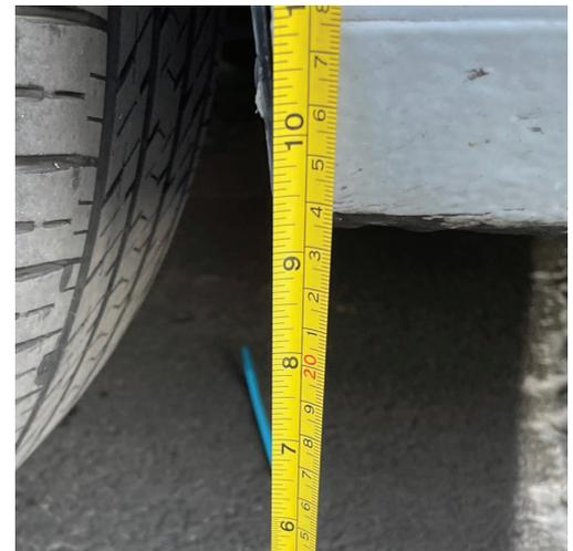
We got around 0.9" ground clearance after installation.
