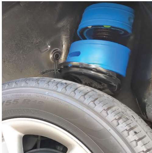
Rear coil springs : DuraTPEPlus A / BP installed
