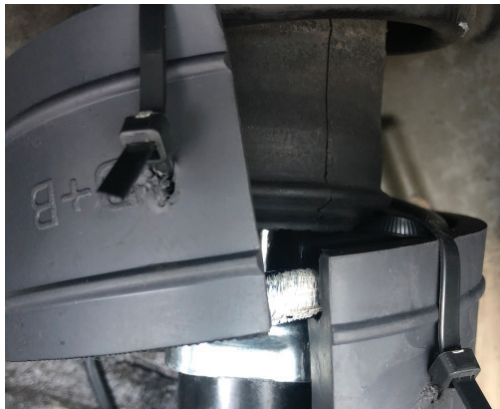
4. ¼" diameter holes are drilled in the center line and 1-2 inches away from the open edges Buffers were tied to the top coil on both end with included zip ties
