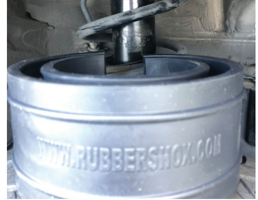
3. Based on the measurement, we can only choose Size B+, H2=1.3". Size A H2 = 1.85 cannot fit into the springs.
