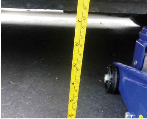
1. Vehicle height before install the buffers and blocks. 7.25"
