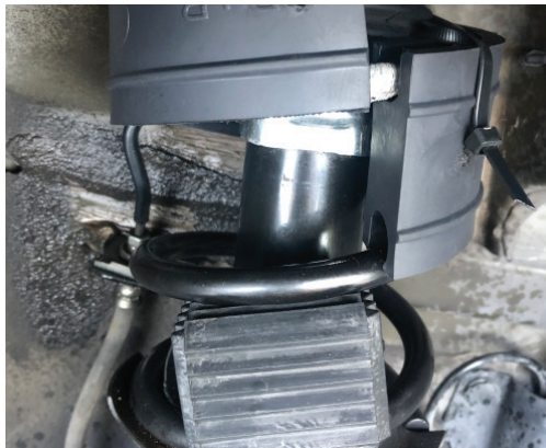
5. Customer want more lift on his car, so Rubber Block Boosters are installed with the buffer. RB2-15-125 blocks were chose to install underneath the opening of the buffers on 1.5" side RB2-15-125 can install on gap, 2", 1.5" and 1.25"
