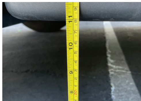
10. Ground clearances increase one inch from 10" to 11"
