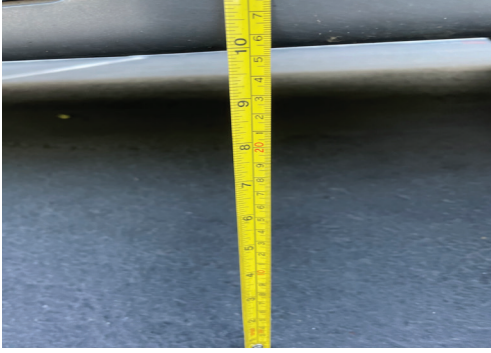
1. Vehicle ground clearance before installation is 10"
