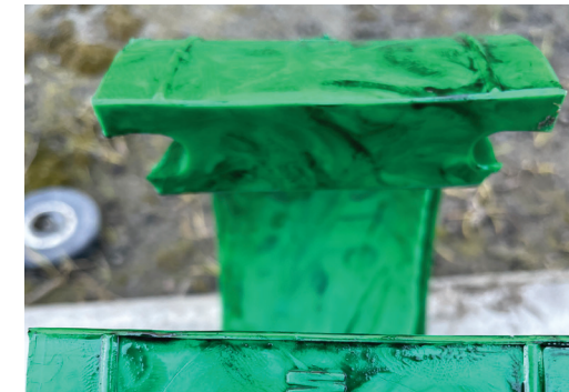
8. Due to the H2=2.36" is very close to Gap of 2.5", Both top and bottom inner rings were trim off.
