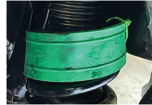
5. Front coil spring buffers installation completed, zip ties included to secure buffer in place.
