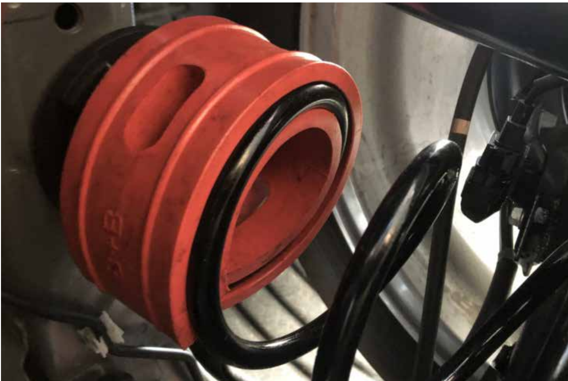
DuraTPE Series Model CSB-BP installed at 2019 Honda CRV Rear Coil Spring.
