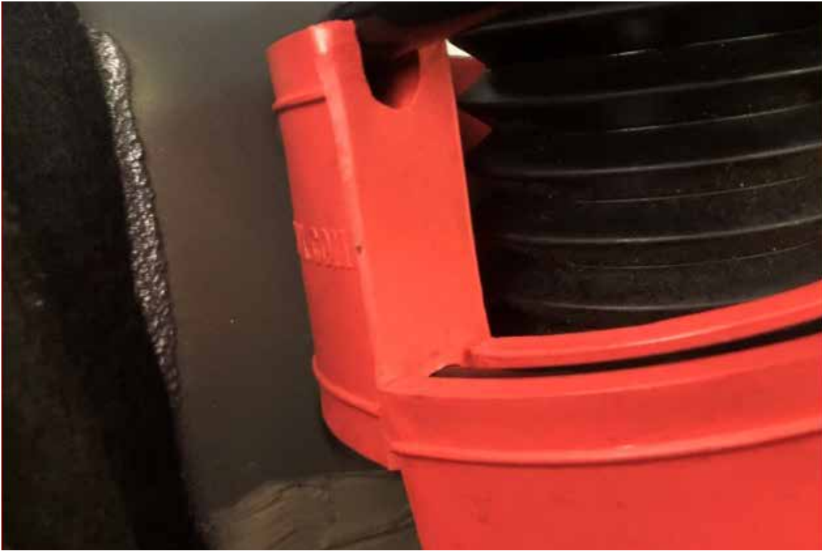
DuraTPE Series Model CSB-AP installed at 2019 Honda CRV both Front Coil Spring.
