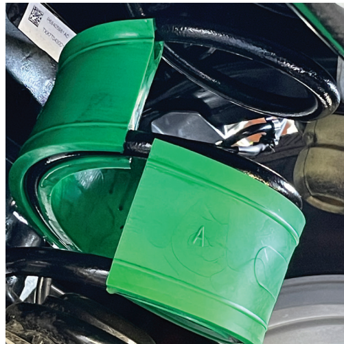
6. CSBSuper-A was selected for the rear coil spring installation
