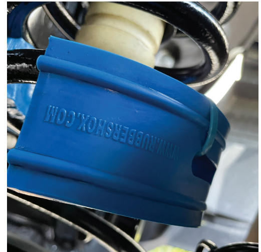
4. After installation of the CSBPlus-C
