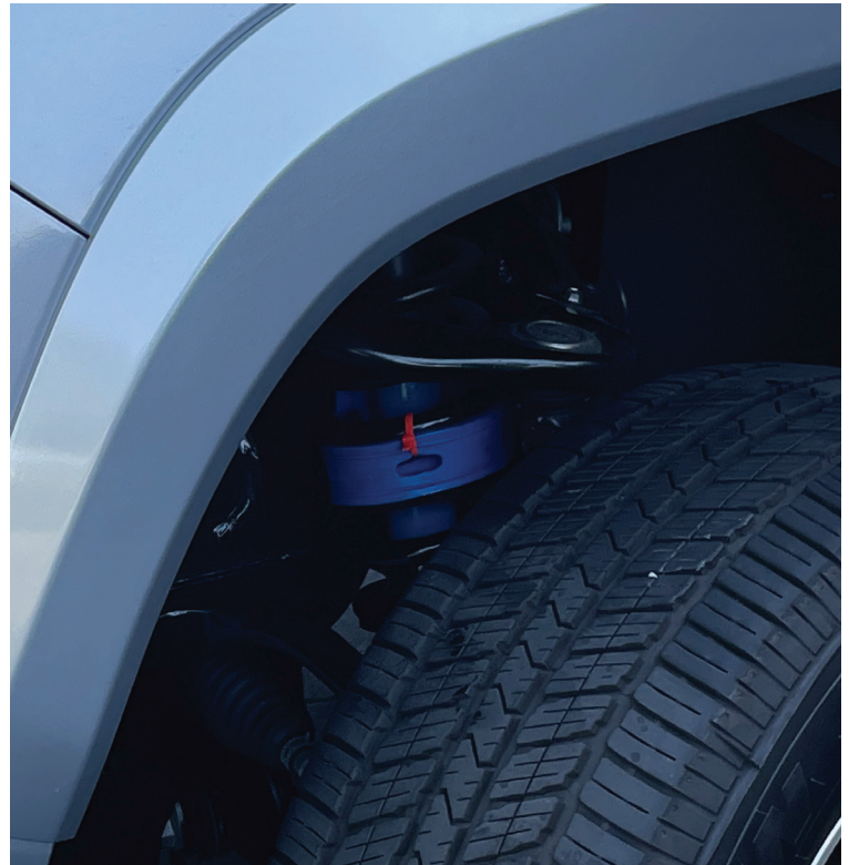
Tight up the buffer on top of the coil spring with included zip ties.
