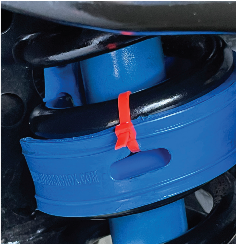
This truck coil spring diameter is too big, so it is very hard to install the buffer. We cut of the top inner ring to ease the installation.
