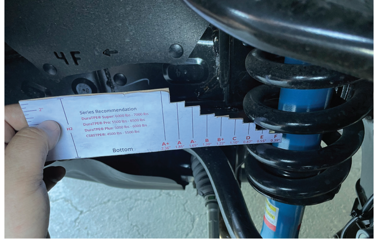
Use the template to choose the correct buffer for the front coil spring after lifting up the truck. It shown size E on the template.
