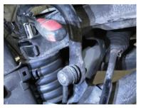
2. Remove UB13 (Left) by using a 17mm Deep Socket Wrench (Installing UB122 on the right using same 17mm deep socket wrench)
