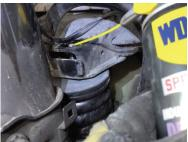
3. Place UB122 and Spray WD40 on SS Stud before insert
