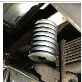
He measured the frame to axel distance is around 6.5" without loading the camper and 3.5" after loading the camper. There is 3 inches drop.
