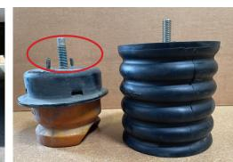
Original F150 factory bump stop VS RubberShox heavy duty natural rubber bump stop UB13
