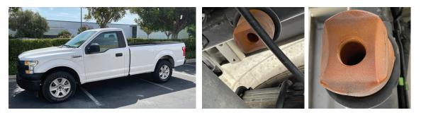
Unload ground clearance: 18 ¾" Rear and 17" front. Original Bump Stop – Cheap synthetic rubber and very tiny. Frame will not hit the bump stop even with 1 ton loading. This will affect the driving condition and cause fish tail in highway speeds.
