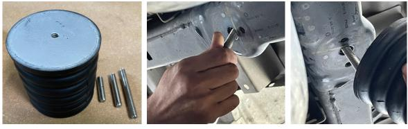
Pick the shortest screw for F150 installation
