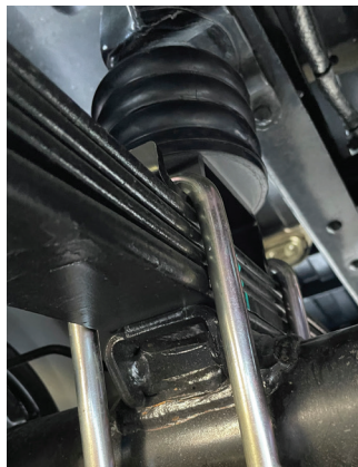
After replaced with UB1+UB2 or our UBS series bump stop. The truck looks flat from front to back with the rear height 35".
