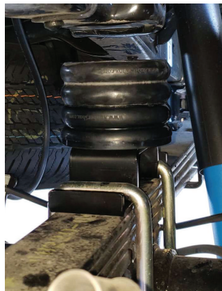
After replaced with UB1+UB2 or our UBS series bump stop. The truck looks flat from front to back with the rear height 35".
