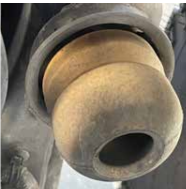
Factory Bump Stop Wears off after 4 years.
