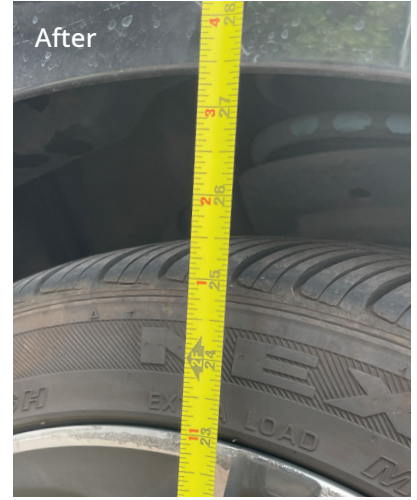
Before installed the modular buffer - Ground clearance 27.5" After installation - Ground Clearance 28.25"
