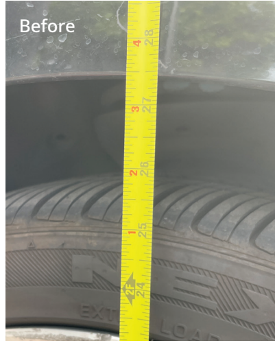
Before installed the modular buffer - Ground clearance 27.5" After installation - Ground Clearance 28.25"
