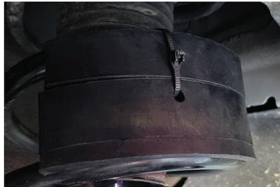
8. There are around 1" ground clearance increase after installed the UCSB buffers
