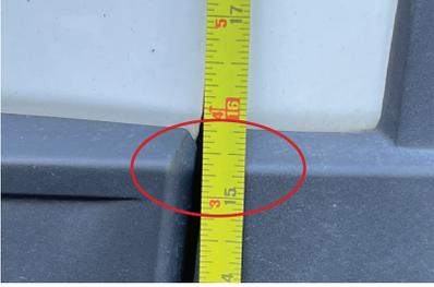
2. Measure the distance between coil spring after jacked up the vehicle
