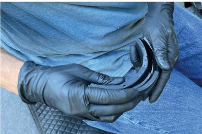
5. Lubricate UCSB1's both grooves and put on top of the coil then put the UCSB2+4 assemble in the bottom of the coil
