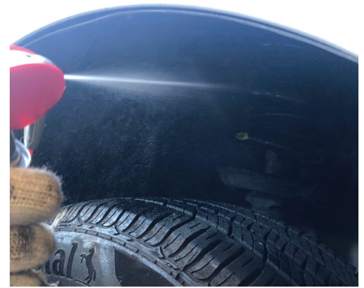
3. Use WD-40 to lube the coil springs. Please spray evenly to coil spring
