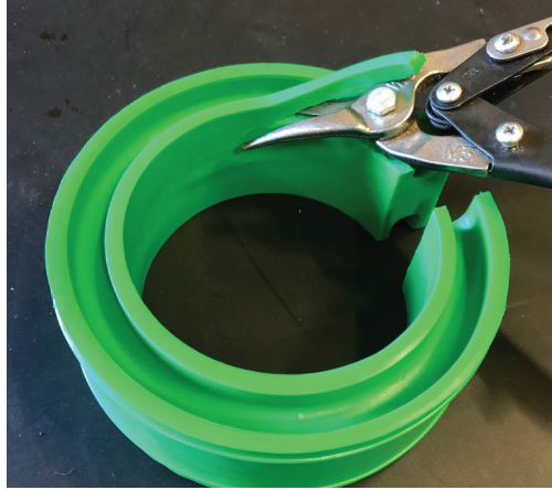
2. Front coil spring gap measured at around 1.3", we pick CSBSuper-B for firm support and maximum lift.
