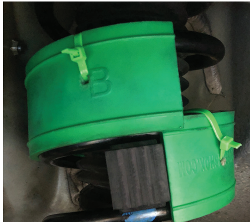
5. For firmest support and lift, we use CSBSupper (70HA) series size B to install on the front coil spring and add Rubber Block Booster RB125-1-1 right under the opening to add more lift and support.
