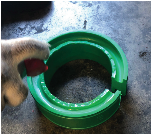
4. Spray WD-40 inside both top and bottom grooves.
