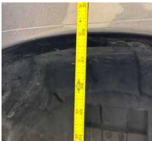
Factory bump stop ground clearance is 38" without any loading on the truck.
