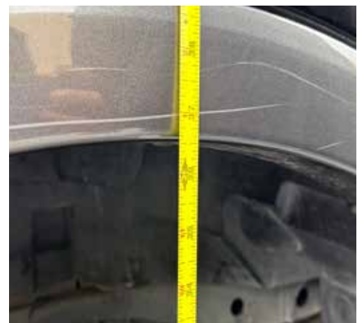
RubberShox MUB1222 (3x MUB2) ground clearance is 36.6" with a 1300 lb load in the truck bed – Almost a 1" increase.
