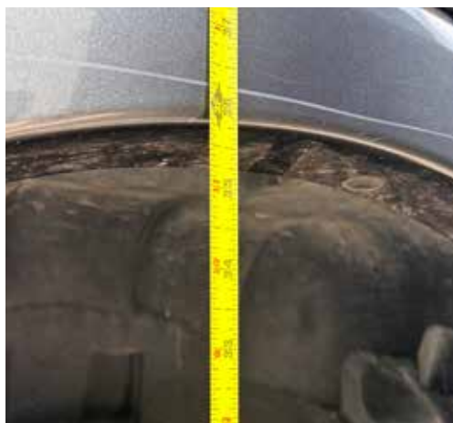
Factory Bump stop ground clearance is 35.75" with a 1300 lb load in the truck bed.
