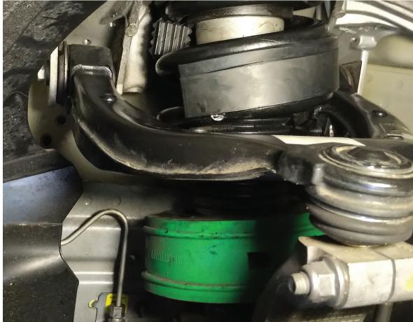
**Tip:** Require Inner Groove Cut for easier install. (CSB Super Item only) (UCSBH12344 is a modular of UCSB1/2/3/4/4 to choose right height to combine to your gap, do not need any cut)
